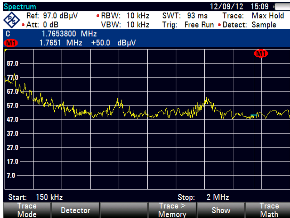
Figure 29. Conducted EMI Pre-compliance 150 kHz–2 MHz
