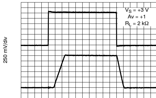
Figure 24. 3 V Non-Inverting Large Signal Pulse Response
