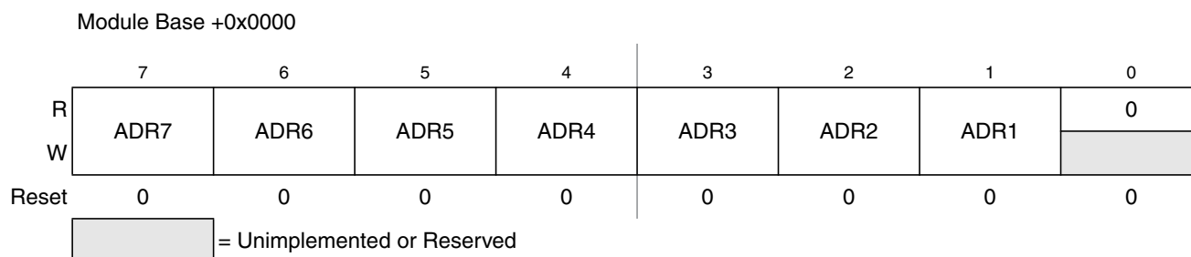
Figure 15-3. IIC Bus Address Register (IBAD)
