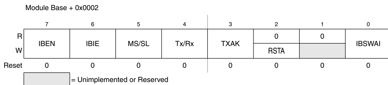
Figure 15-6. IIC Bus Control Register (IBCR)
