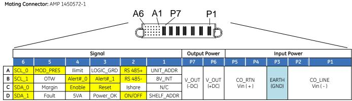
Connector is viewed from the rear positioned inside the power supply.
