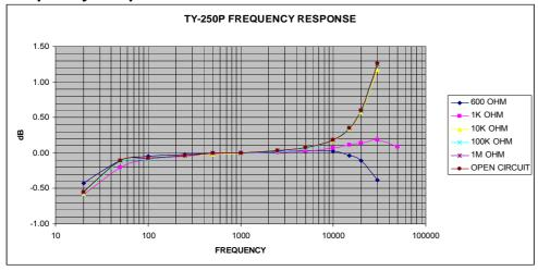
\* 600:600Ω, 10K:10KΩ, 100K:100KΩ, 1M:1MΩ, and other impedances (secondaries can all be used at  $\frac{1}{4}$  value when placed in parallel) are optional as long as input voltage is  $\leq$ 4.2Vrms and current is  $\leq$ 7mA.
