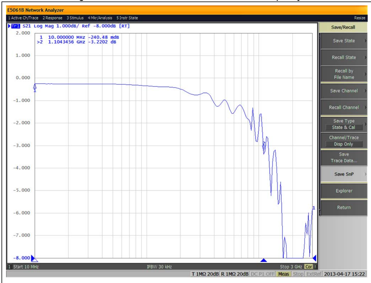
Figure 22. Data switch transfer characteristics vs. frequency
