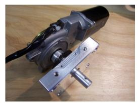
**Step 4:** Insert the three M4 x 50 mm socket-cap screws into the counter-sunk holes as shown. Slide three 1'' long standoffs onto the screws and then line up the screws to the motor screw holes and tighten with a 5/32'' Allen wrench.
