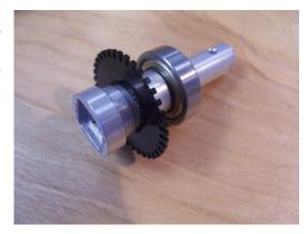
**Step 2:** Insert the axle assembly into the Bearing Block. This will be a very close tolerance fit. Take care to properly align the bearing with the block while maintaining a gentle pressure. Very gentle tapping with a wooden mallet can be used if required. This close-tolerance fit is by design.
