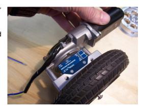
Step 13: Gently spin the wheel assembly, and watch how the encoder disk spins in relation to the encoder's slot. Adjust the disc such that it spins freely within the confines of the Encoder's slot.
