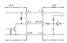
Note: The PLC connects to the M7F with ease via the G79-O□C-□ Cable (with connectors, sold separately). (The above example indicates 1 to 1 connection.)
