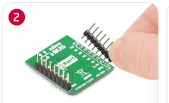
Turn the board upside down to face its bottom side. Place shorter parts of the header pins in both soldering pad locations.
