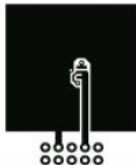
a. 78 ^{\circ}\text{C}/\text{W} when mounted on a 1 in 2 pad of 2 oz copper
