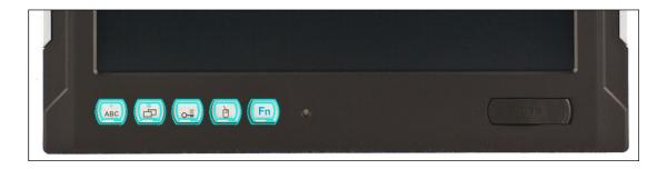
Depending on the equipment version, an operating system and a soft keyboard has previously been installed ex works. The keys on the front panel are occupied with the following functions by a specific driver in the soft keyboard:
