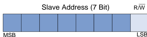
Figure 9.3 Control Byte Format.
