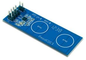
the PmodCDC1 to adapt its threshold level. The adaptive threshold is a programmable feature of the AD7156.
