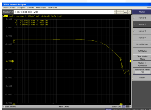
Figure 17. MHL Path SDD21 Insertion Loss Curve
