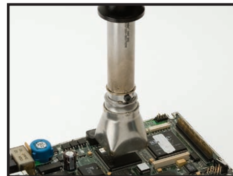
Efficiently desolders QFP's and other SMT components
