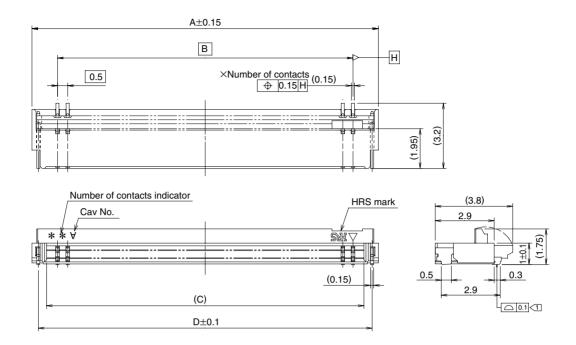
Note 1: The coplanarity of each terminal lead within specified dimension is 0.1 mm Max.
