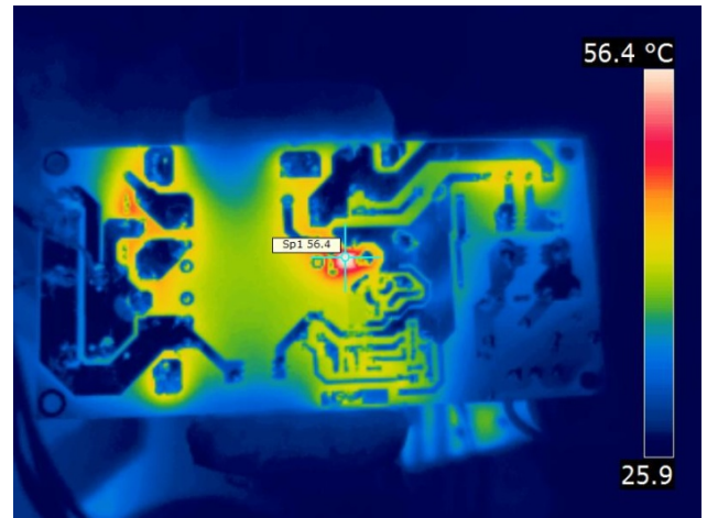
Figure 19 – Blocking Diode D4 (Sp1) Case Temperature.
