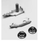
The 4460-D Shield Bond Connector is a downsized version of the 4460 Shield Bond Connector. Its small size makes it an excellent choice for cables of 100-pair or less. Its current-carrying capacity is equal to or better than aluminum-shielded cables of 100-pair or less and can be used on all cable with 20.3 mm (0.8") or smaller O.D.
