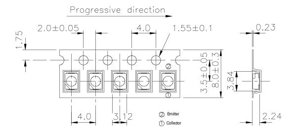
TOLERANCES UNLESS DIMENSION±0.1 ANGLE±0.5 UNIT:mm
