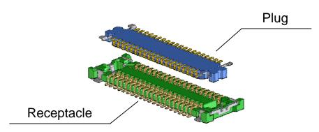
The AA01A Series connectors are 0.5mm-pitch, stacking type, board-to-board connectors ideal for slim, low-profile devices such as mobile phones, LCDs, notebook PCs, and PDAs, which have high density mounting requirements.
