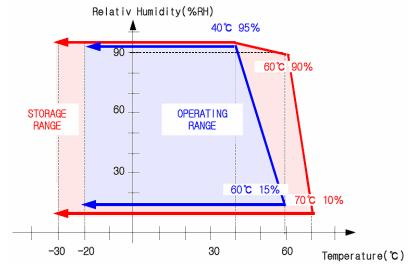
(2) In case of below 0°, the response time of liquid crystal (LC) becomes slower and the color of panel becomes darker than normal one. Level of retardation depends on temperature, because of LC's character
