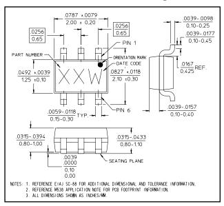
Reference Application Note M538 for lead-free solder reflow recommendations.
