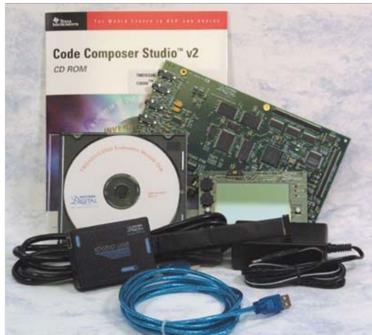
EVM320VC5502 + Keypad/display Module + Power Supply + XDS510 USB Emulator + Code Composer Studio Platinum
