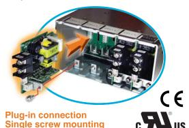
The C Series power supplies save design and production time and cost by allowing end-of-line selection of multiple output voltages to match alternative application circuit requirements, while using the same power supply base unit. DC voltage output modules are slot-mounted inside the base units to provide various combinations of single, dual, or parallel output voltages.
