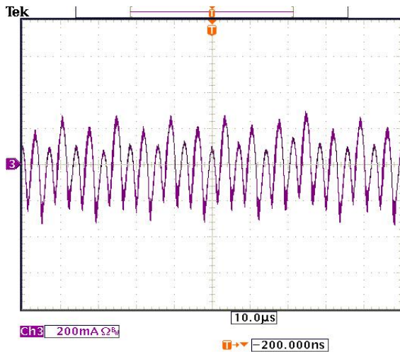
Figure 9: Input Terminal Ripple Current, i_c , at nominal input voltage and rated load current with 12\mu\text{H} source impedance and 150\mu\text{F} electrolytic capacitor ( 200\text{ mA/div} ).
