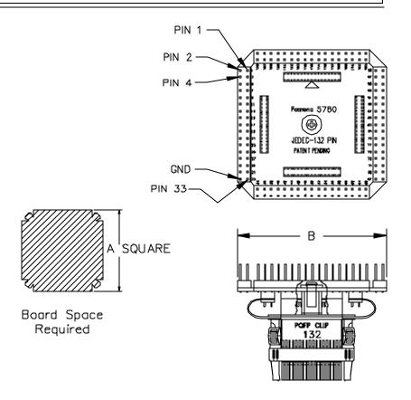
The patented locking mechanism holds the clip on the device by gripping the chip body at the end of each lead pattern. Each contact is individually cantilevered to assure positive contact. Three other types of interfaces are available for connection to your instruments. See Pomona's full line catalog for complete details. Other clips are available in many sizes to fit the most popular chips now in use.
