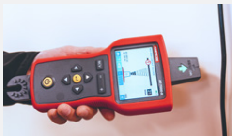
Non-contact voltage (NCV) detection.
