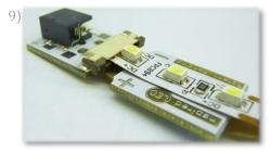
Reinforce the connection by pressing and sticking the flexible strip to the rest of the connector board.
