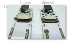
Also notice the LED connector - it opens for easy strip insertion and latches to secure the connection.
