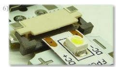
Insert the flexible LED strip into the open LED connector: above the sliding latch and below the beige top. Again, make sure that the positive side of the strip matches the positive side of the board.
