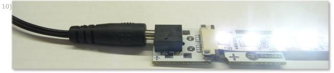
If there is any flickering, make sure flex is fully inserted and that the latch is secure. If no lights turn on, check polarity.
