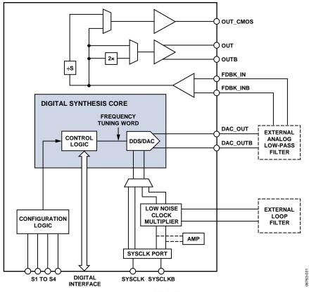
Figure 39. Detailed Block Diagram
