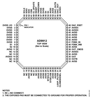
Figure 2. Pin Configuration
