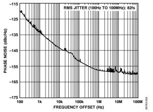
Figure 25. Absolute Phase Noise of Unfiltered DAC Output, f<sub>OUT</sub> = 311.6 MHz, SYSCLK Driven by a 1 GHz Wenzel Oscillator (SYSCLK PLL Bypassed)
