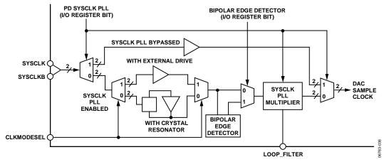
Figure 44. System Clock Generator Block Diagram
