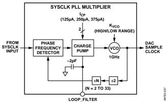
Figure 45. Block Diagram of the SYSCLK PLL
