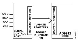
Figure 50. Relationship Between Serial Control Port Register Buffers and Control Registers of the AD9912
