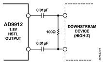
Figure 33. AC-Coupled HSTL Output Driver
