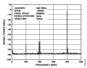
Figure 8. Wideband SFDR at 398.7 MHz, SYSCLK = 1 GHz (SYSCLK PLL Bypassed)
