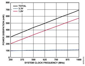
Figure 18. Power Dissipation vs. System Clock Frequency (SYSCLK PLL Bypassed), f<sub>OUT</sub> = f<sub>SYSCLK</sub>/5, HSTL Driver On, CMOS Driver On, SpurKiller Off
