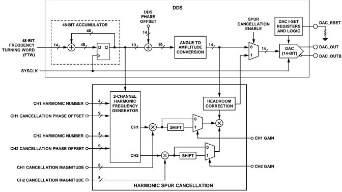
Figure 48. Spur Reduction Circuit Diagram
