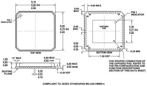
Figure 57. 64-Lead Lead Frame Chip Scale Package [LFCSP\_VQ] 9 mm × 9 mm Body, Very Thin Quad (CP-64-7) Dimensions shown in millimeters
