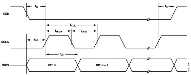
Figure 56. Serial Control Port Timing—Write
