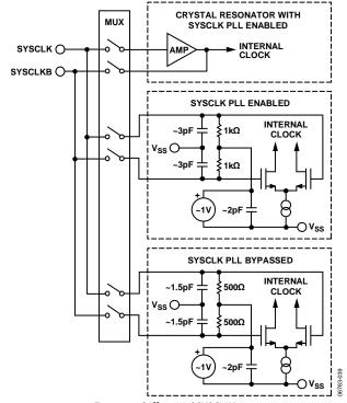
Figure 47. Differential SYSCLK Inputs
