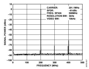
Figure 7. Wideband SFDR at 201.1 MHz, SYSCLK = 1 GHz (SYSCLK PLL Bypassed)
