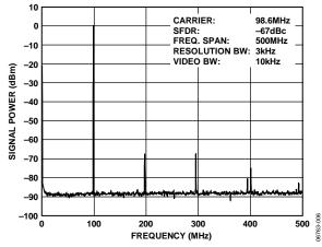
Figure 6. Wideband SFDR at 98.6 MHz, SYSCLK = 1 GHz (SYSCLK PLL Bypassed)
