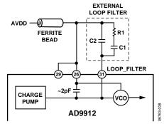
Figure 46. External Loop Filter for SYSCLK PLL
