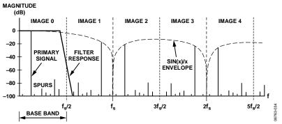
Figure 42. DAC Spectrum vs. Reconstruction Filter Response
