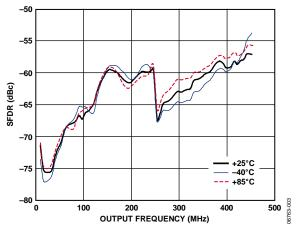
Figure 3. Wideband SFDR vs. Output Frequency at  $-40^{\circ}$ C,  $+25^{\circ}$ C, and  $+85^{\circ}$ C, SYSCLK = 1 GHz (SYSCLK PLL Bypassed)
