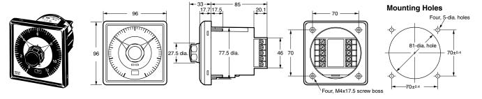
Note: Tightening torque for panel mounting is as follows: 300 m N·m ±50 m N·m
