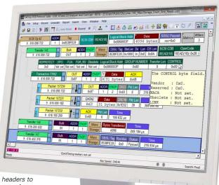
The CATC Trace display uses collapsible headers to group all packets that are part of a single transfer
