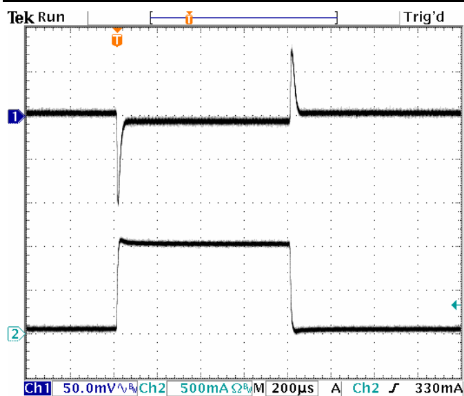
Load Transient: V_{IN} = 3.7V , V_{OUT} = 1.2V Load stepped from 0mA to 1000mA
