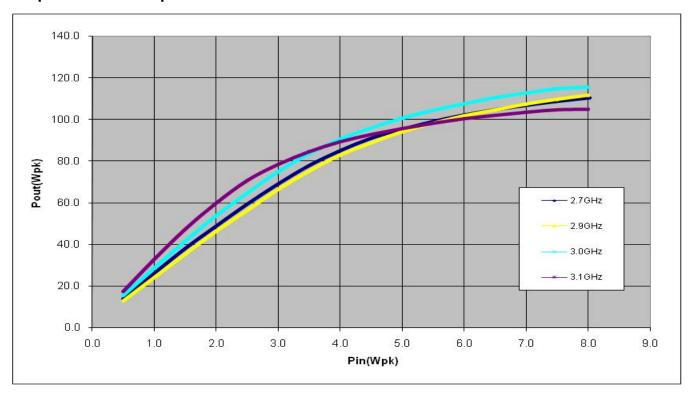
Gain vs. Frequency 50V Drain Bias, Idq=0.5A
