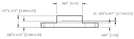
Unless otherwise noted, tolerances are inches  $\pm .005$ " [millimeters  $\pm 0.13$ mm]
