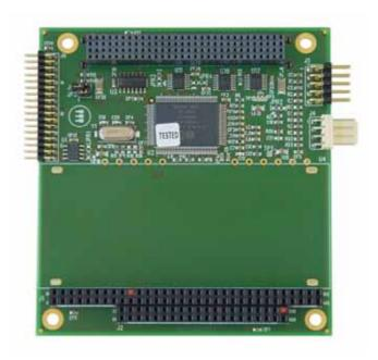
The INT-1462 video frame grabber is a cost-effective, high-performance solution for capturing analog broadcast signals across the PCI bus. Based around the Conexant Fusion™ 878A video decoder, this compact PC/104-Plus form factor board supports NTSC, PAL, and SECAM video formats at capture resolutions of up to 768x576 pixels and 30 frames per second. It also has the ability to sub-sample, scale, crop, and clip images at various resolutions and frame rates.
