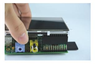
**NOTE:** The 4DPi-35 is supported only by the 26 way header, and therefore pressing on the touch screen may result in the 4DPi-35 moving towards the Raspberry Pi, and therefore the circuitry touching the Raspberry Pi. This could result in damage to either product if a short circuit were to occur. It is therefore highly encouraged to mount the display and attach the Pi to the mounted display.
