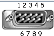
RS-232 Pin-out DB9 Male DTE
