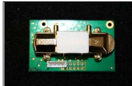
Figure 5: T6613/6615 CO 2 Sensor with 4 Pin Header
