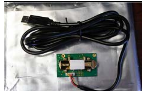
Figure 6: T6613/6615 CO 2 Sensor Connected to USB Cable
