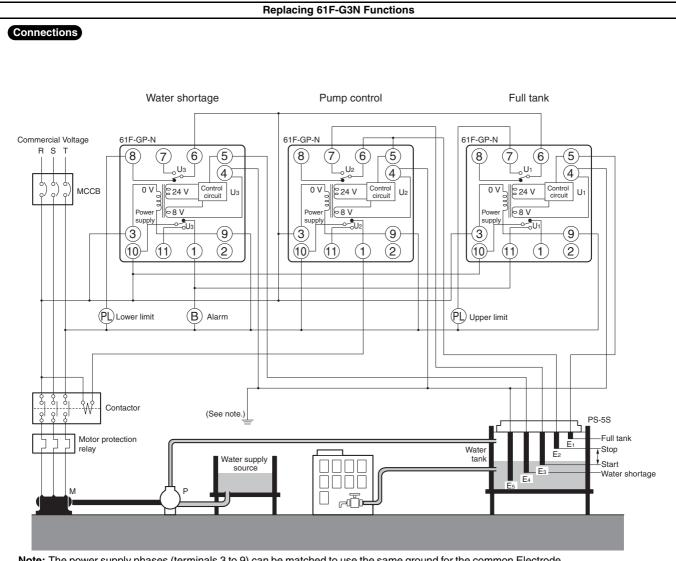
Note: The power supply phases (terminals 3 to 9) can be matched to use the same ground for the common Electrode (the longest Electrode, terminal 4).
