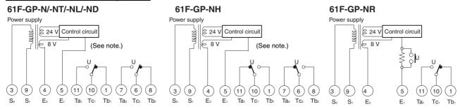
Note: When applying a self-holding circuit, short between terminals 5 and 6 and use terminal 7 as  $E_2$ .
