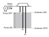
The pump stops when the water level reaches E<sub>1</sub> (indicator ON) and starts when the water level drops below E<sub>2</sub> (indicator OFF).
