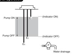
The pump starts when the water level reaches E<sub>1</sub> (indicator ON) and stops when the water level drops below E2 (indicator OFF).
