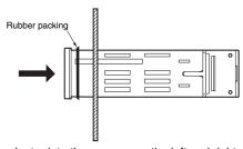
Fit the adaptor into the grooves on the left and right sides of the rear case, then push it until it contacts the panel to secure the K3MA-J.
