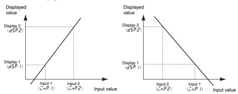
Instead of setting by inputting with the Shift Key and Up Key, current measurement values van be input as scaling input values for teaching. This is useful for making settings while checking the operation status of the K3GN.
