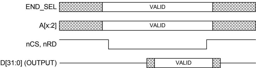
Figure 8.3 Functional Timing for PIO Read Operation
