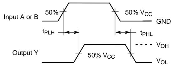
**Figure 4. Switching Waveforms**
