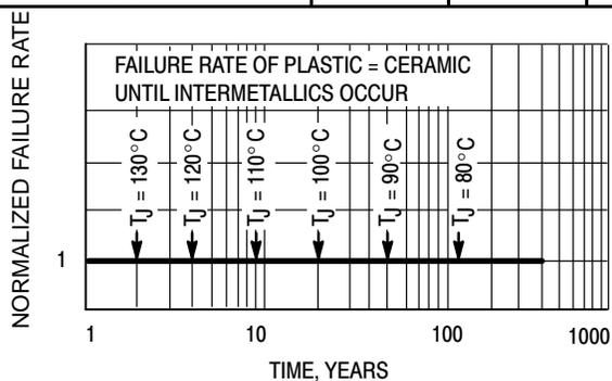
Figure 3. Failure Rate vs. Time Junction Temperature
