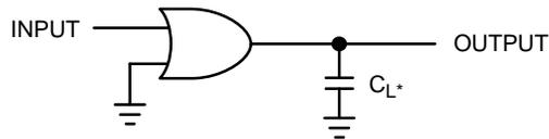
\*Includes all probe and jig capacitance.
