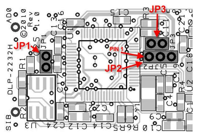
The mode select jumpers (**JP1 – JP3**) are identified above and on the silkscreen. They are located in the center and top of the DLP-2232H module. These three jumpers control the usage of the DLP-2232H module's pins 17 and 18 as follows:
