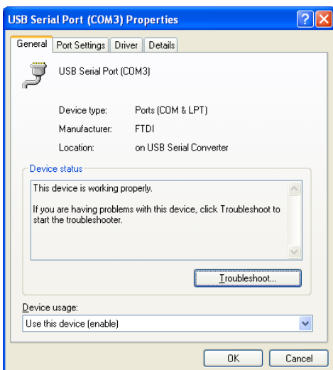
Figure 3-9 Access COM Port Properties
