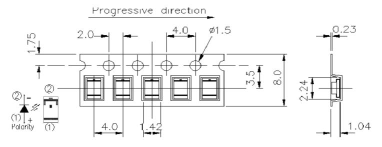
**Note:** The tolerances unless mentioned is  $\pm 0.1$ mm, Unit = mm
