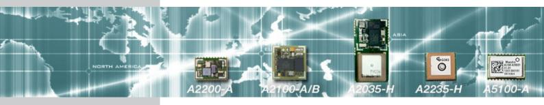
The A5100-A module is housed in a 15.0 x 10.2 x 2.5mm 22-pin SMD package with castellated edge that includes all RF matching elements, antenna DC control, RF SAW filtering, various thermal and peripheral components and the TCXO crystal reference.
