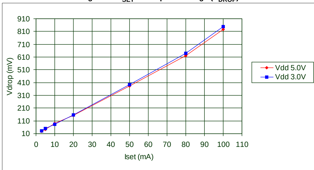
Figure 12. I_{SET} vs drop out voltage ( V_{DROP} )
