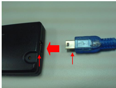
Figure 2-14: Connect the USB cable to the Logic Analyzer
