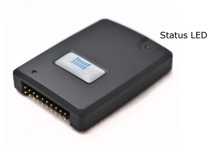
Figure 1-2: Logic Probe connections (ES-DLA-16 shown) and Status LED
