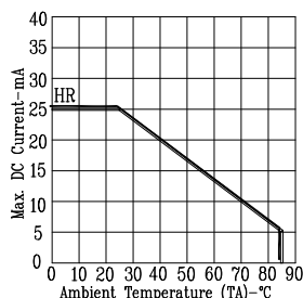
Fig5. MAX. ALLOWABLE DC CURRENT VS. AMBIENT TEMPERATURE.
