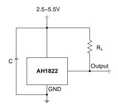
Notes: 4. C is for power stabilization and to strengthen the noise immunity, the recommended capacitance is 10nF-100nF. R<sub>L</sub> is the pull-up resistor, the recommended resistance is  $10K\Omega$ - $100K\Omega$ .
