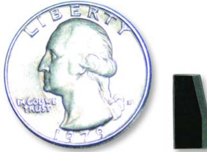
Figure 3-6. The Atmel TK5551M-PP (Atmel ATA5577M1330C-PP) Transponder
